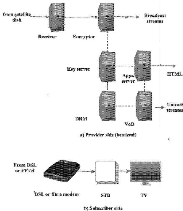
Figure 2 Functional diagram of an IPTV system
